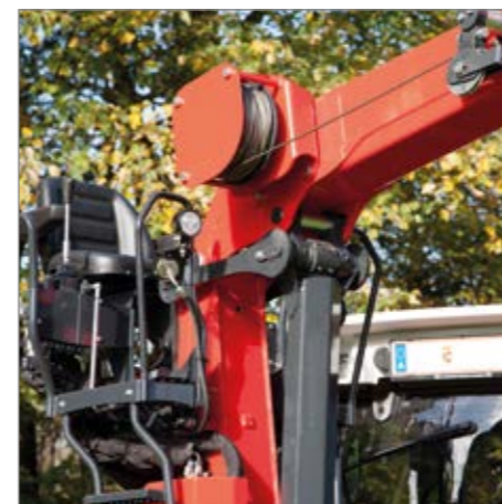
Logging winch (optional) 7mm-thick and 40m-long cable with tensile force of 1.5 t
