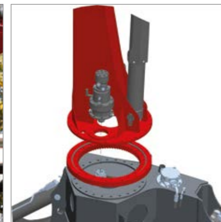
Ball slewing ring Tractor cranes have a crane column with a hardened ball rim bearing and slew transmission inclusive of brake.
