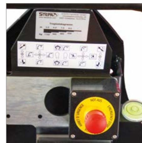
EMERGENCY STOP mechanism always within reach
