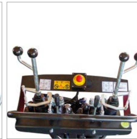
Rotary level two-circuit control system
